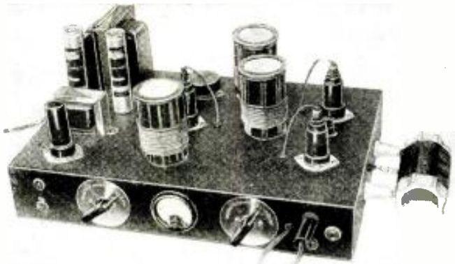
Note the "Prof." appearance of the "R.E.C." transmitter built by Mr. Abrams from receiver parts and tubes.
